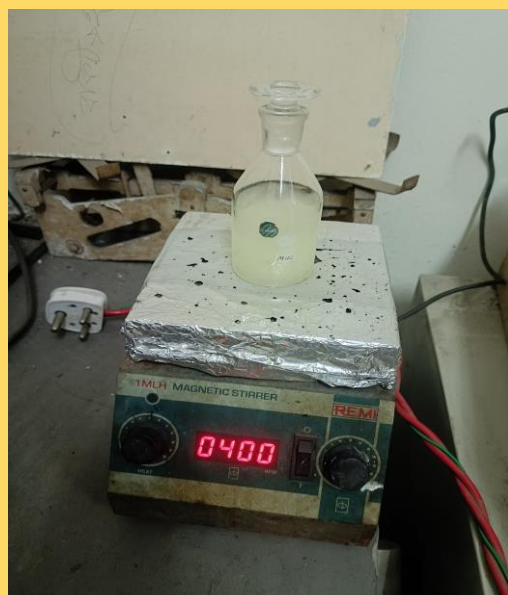
Figure 6: Magnetic stirrer with methanol diesel blend
