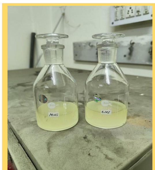
Figure 9: Carbinol (C10%) & Methanol (M10%) mixer with diesel after blending
