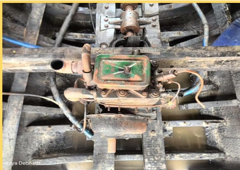
Figure 23: Top view of experimental boat engine 7.5HP
