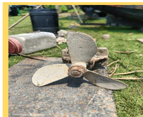
Figure 26: Single screw 3 bladed, Fixed pitch
