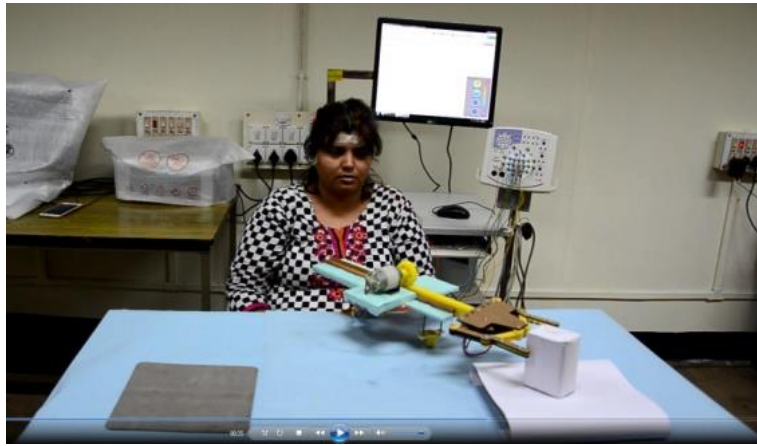
Fig 3.14 Single link position control using motor M_1 of Fig 3.13
