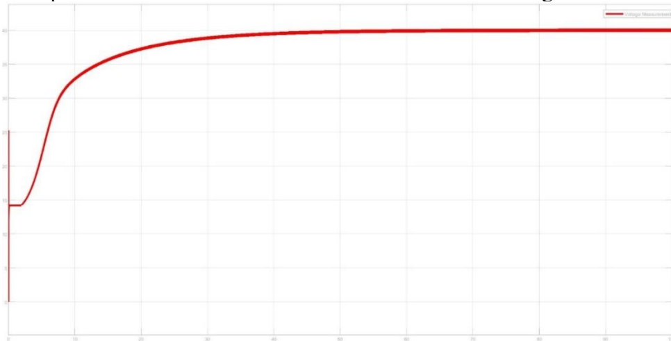
Fig.25: Response of Simscape model of double-loop pi compensation of boost converter
