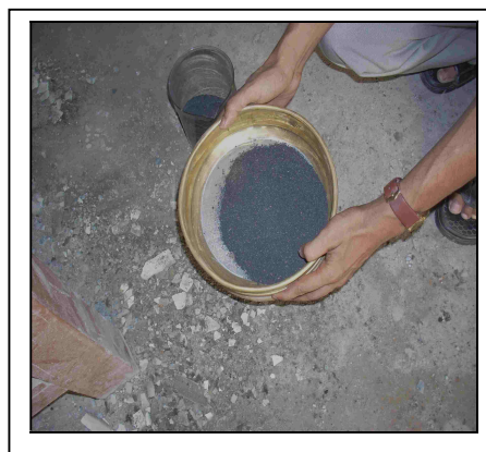
Fig.4.3: Sieving of burnt adsorbent materials with 300 µm sieve
