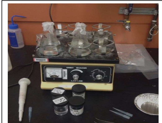
Fig. 4.7: Batch reactor conducting batch study
