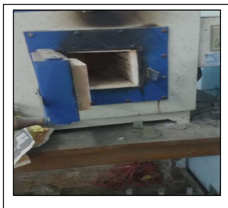
Fig.4.2: Muffle furnace for carbonization of adsorbents
