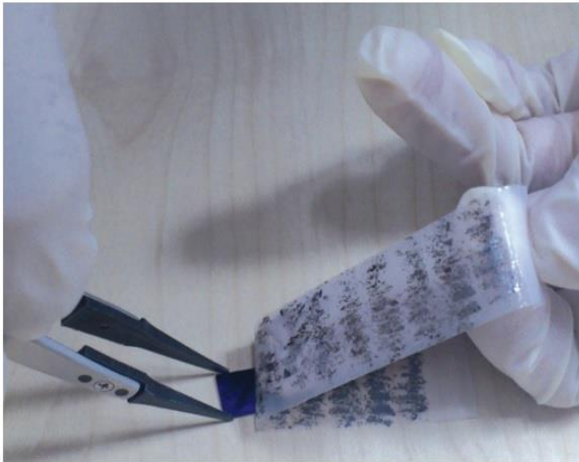
Fig 3.18: [110] Graphene exfoliation by adhesive tape.
