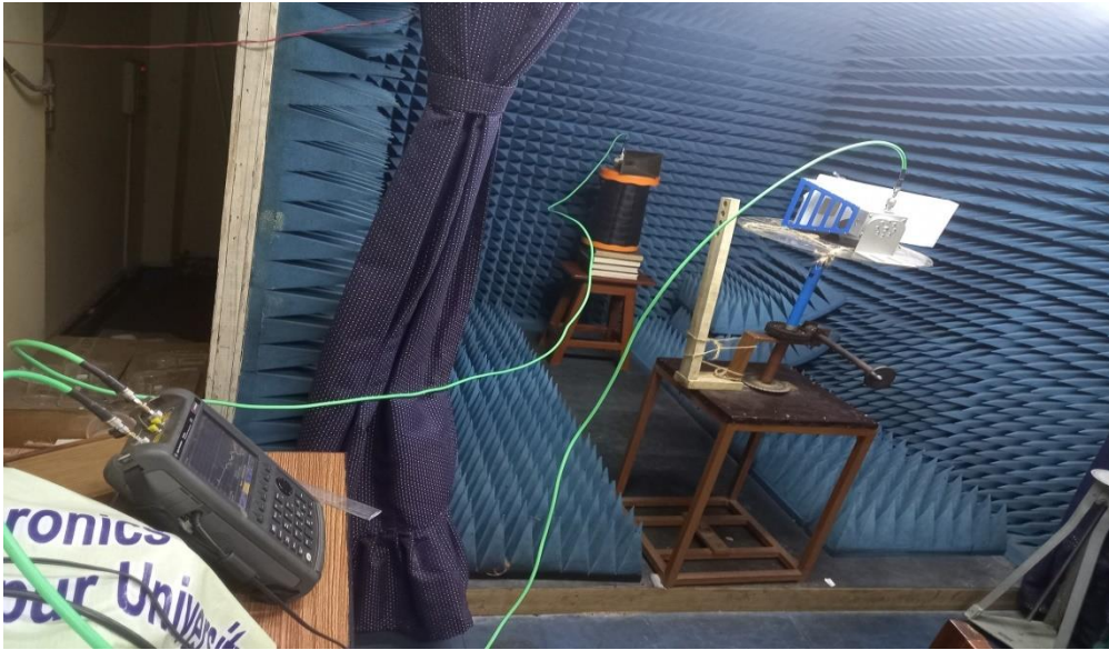
Fig 5.12: Measurement setup of FSS.
