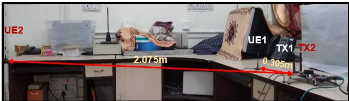
Fig.6.11: Experimental Setup of Downlink two-user (2x2)-MIMO-PD-NOMA model at distance combination A
