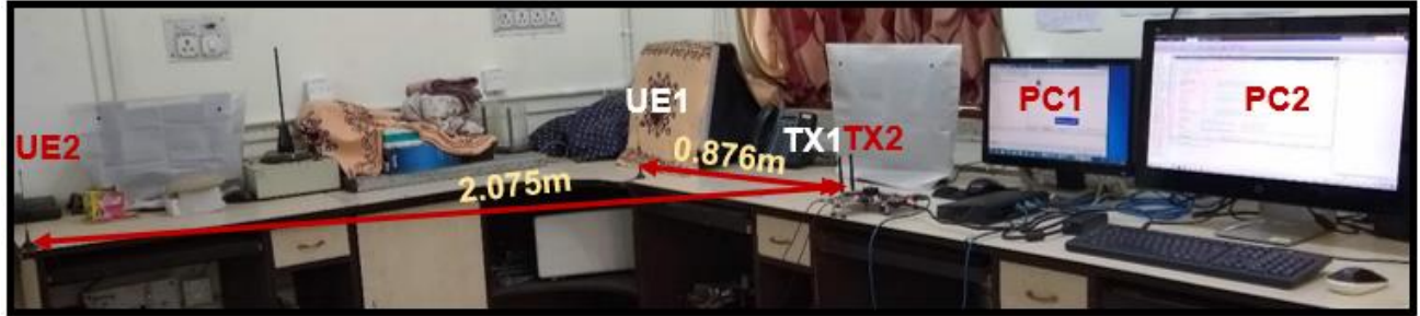
Fig.6.12: Experimental Setup of Downlink two-user (2x2)-MIMO-PD-NOMA model at distance combination B
