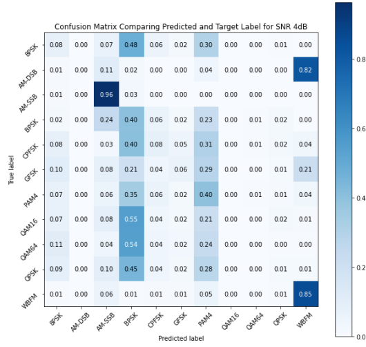
Fig. 3.7 Confusion matrix of CNN based AMC with 3 convolution layers for 4 dB SNR in 1 epoch
