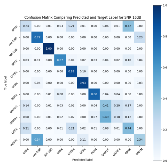
Fig. 3.39 Confusion matrix of CNN based AMC with 4 convolution layers for 16 dB SNR in 10 epochs
