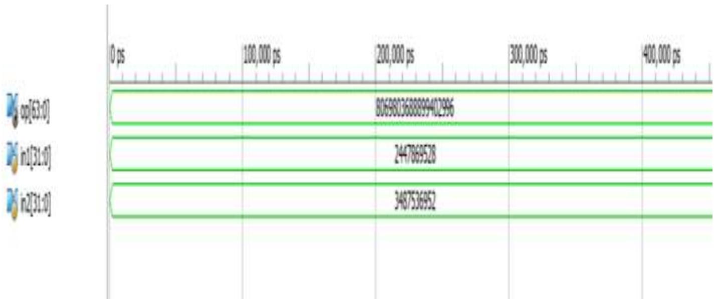
Fig 24: Waveform: 32-bit Approximate Multiplier (Modified)
