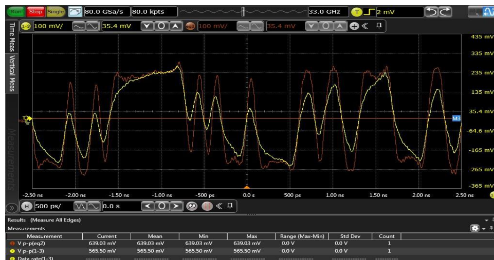
Fig. 6.12. Time domain waveform observed before applying FFE (in yellow) and after applying FFE (in red) for -14dB channel loss.
