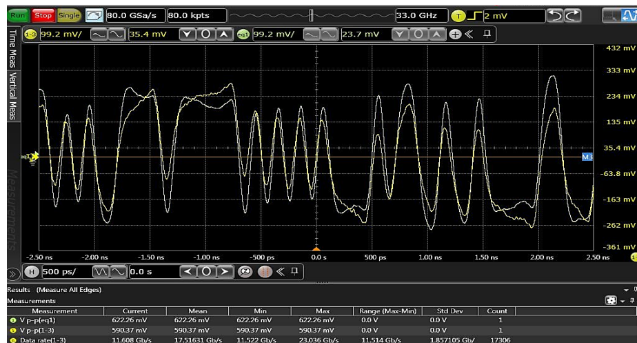
Fig. 6.6. Time domain waveform observed before applying CTLE (in yellow) and after applying CTLE (in green) for -10dB channel loss.
