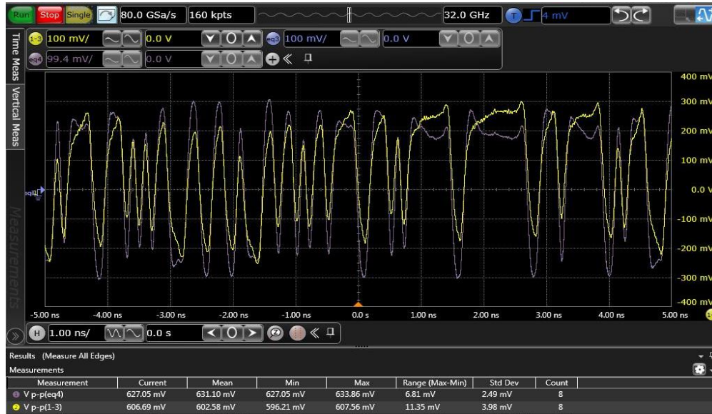
Fig. 6.26. Time domain waveform observed before applying CTLE, FFE & DFE (in yellow) and after applying CTLE, FFE & DFE (in purple) for -10dB channel loss.
