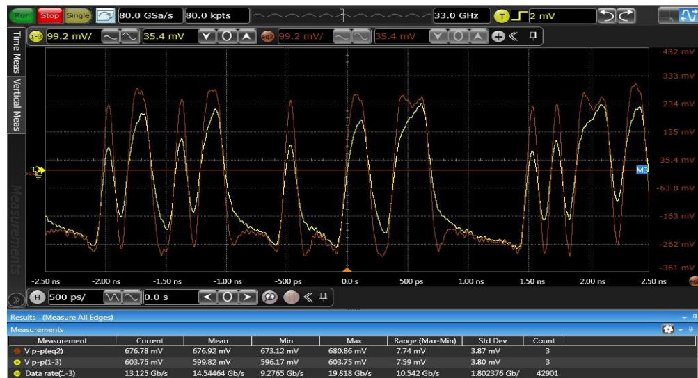
Fig. 6.10. Time domain waveform observed before applying FFE (in yellow) and after applying FFE (in red) for -10dB channel loss.
