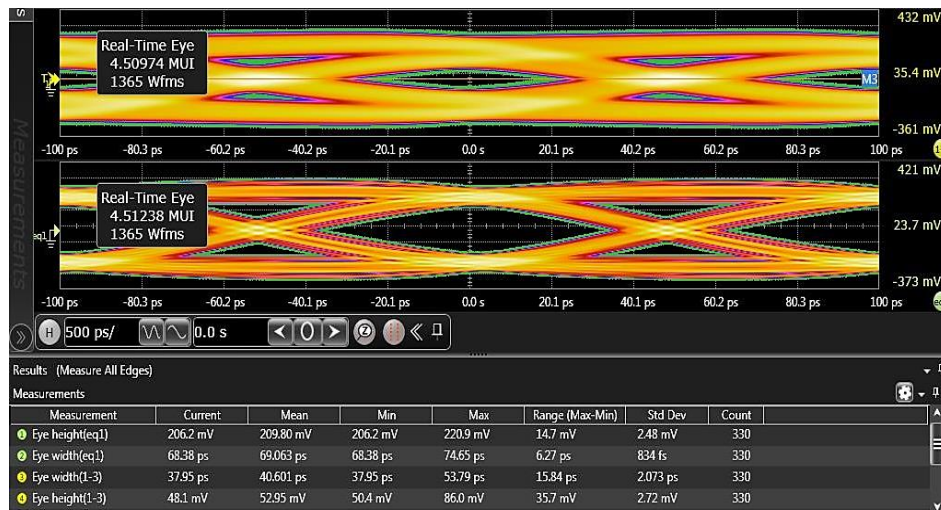
Fig. 6.5. Eye-diagrams observed before applying CTLE (top) and after applying CTLE (bottom) for -10dB channel loss.
