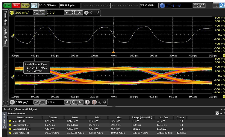
Fig. 6.4. Time domain waveform and eye diagram of the signal travelling through a loss-less channel as observed at receiver (RX) end.
