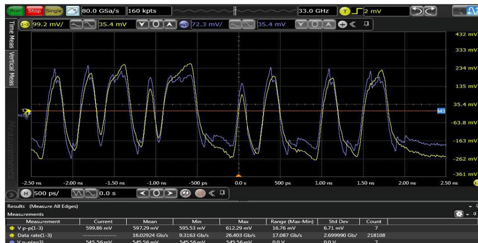
Fig. 6.14. Time domain waveform observed before applying DFE (in yellow) and after applying DFE (in blue) for -10dB channel loss.
