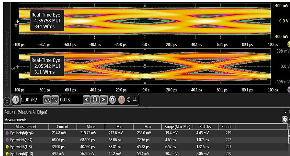
Fig. 6.25. Eye-diagrams observed before applying CTLE, FFE & DFE (top) and after applying CTLE, FFE & DFE (bottom) for -10dB channel loss.
