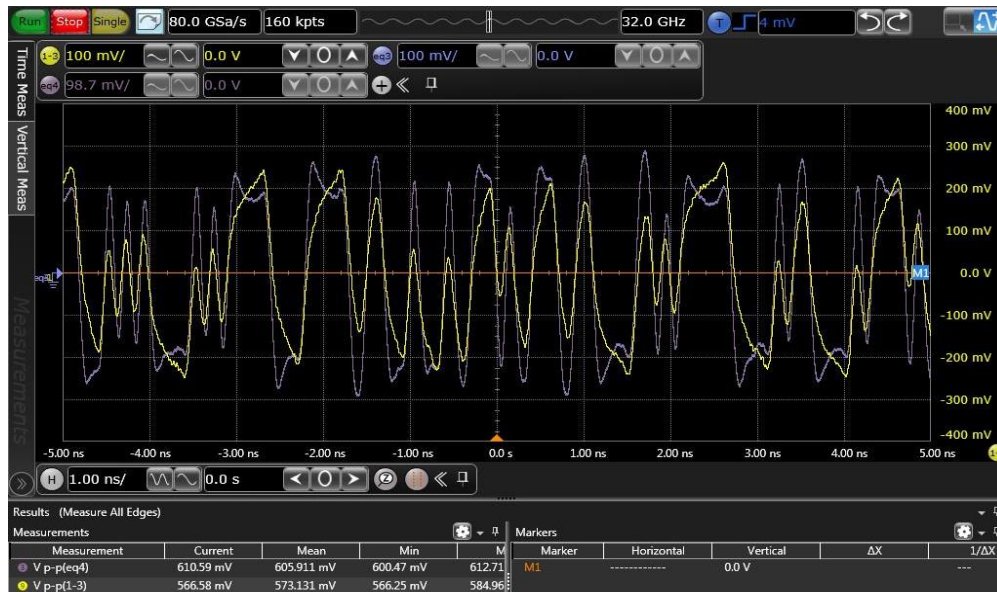
Fig. 6.28. Time domain waveform observed before applying CTLE, FFE & DFE (in yellow) and after applying CTLE, FFE & DFE (in purple) for -14dB channel loss.
