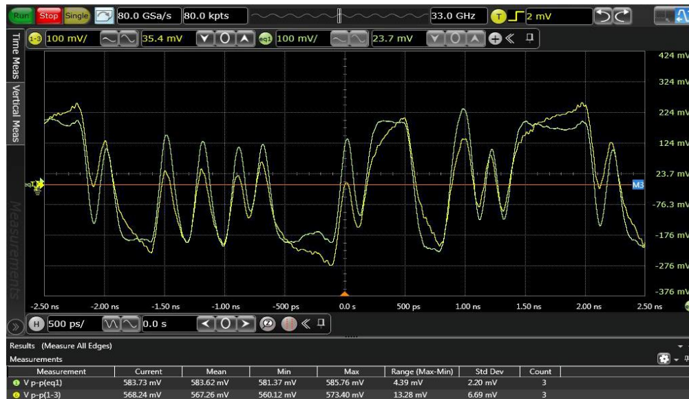
Fig. 6.8. Time domain waveform observed before applying CTLE (in yellow) and after applying CTLE (in green) for -14dB channel loss.
