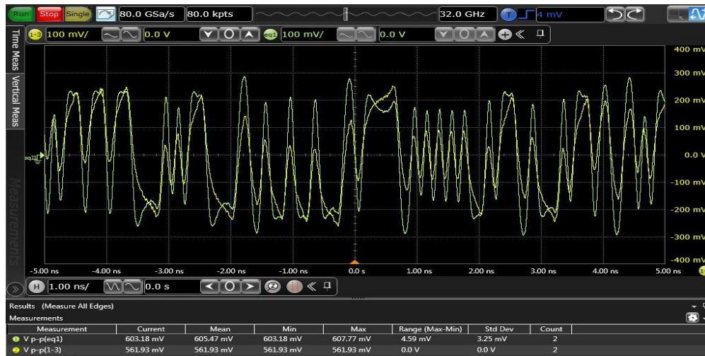
Fig. 6.20. Time domain waveform observed before applying CTLE & FFE (in yellow) and after applying CTLE & FFE (in green) for -14dB channel loss.
