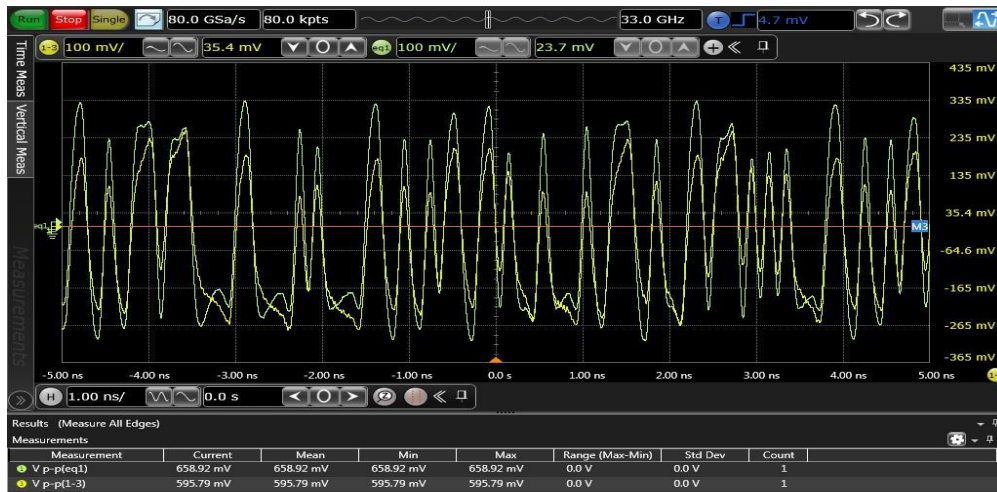
Fig. 6.18. Time domain waveform observed before applying CTLE & FFE (in yellow) and after applying CTLE & FFE (in green) for -10dB channel loss.
