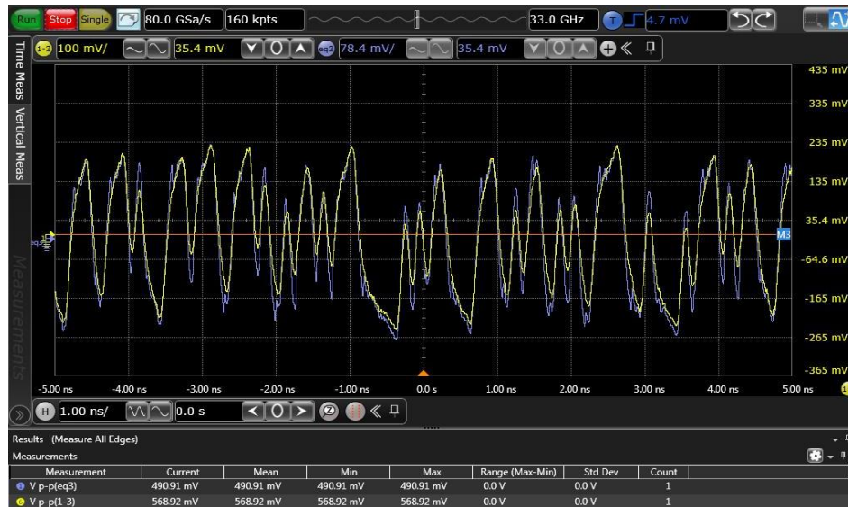
Fig. 6.16. Time domain waveform observed before applying DFE (in yellow) and after applying DFE (in blue) for -14dB channel loss.
