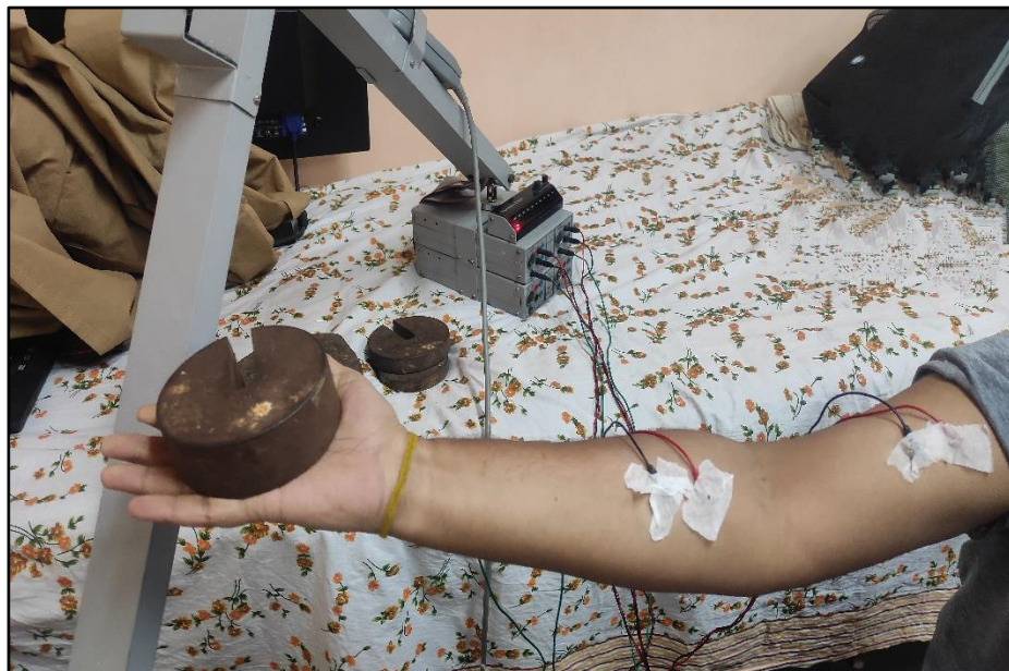
Figure 9: Acquisition of sEMG during static holding fatigue with weight
