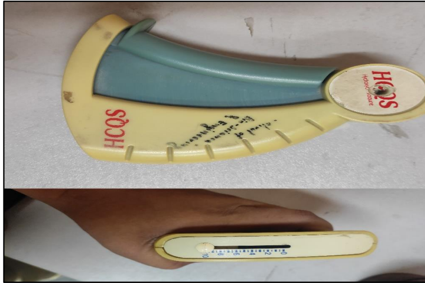
Figure 10: Hand dynamometer used in handgrip fatigue for acquisition of sEMG
