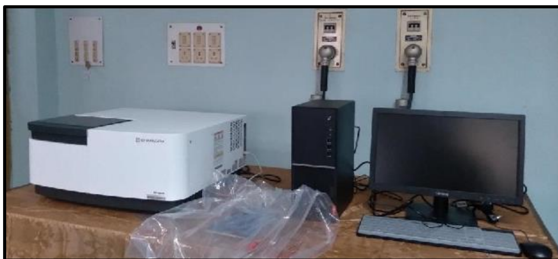
Fig. 3.22: Photoluminescence analysis carried out by Horiba Jobin Yvon Fluoromax
