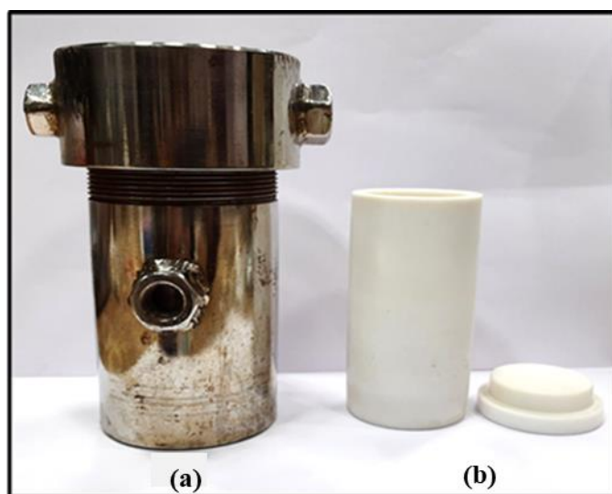
Fig. 3.1: Digital image of (a) autoclave setup and (b) the teflon tube in the autoclave
