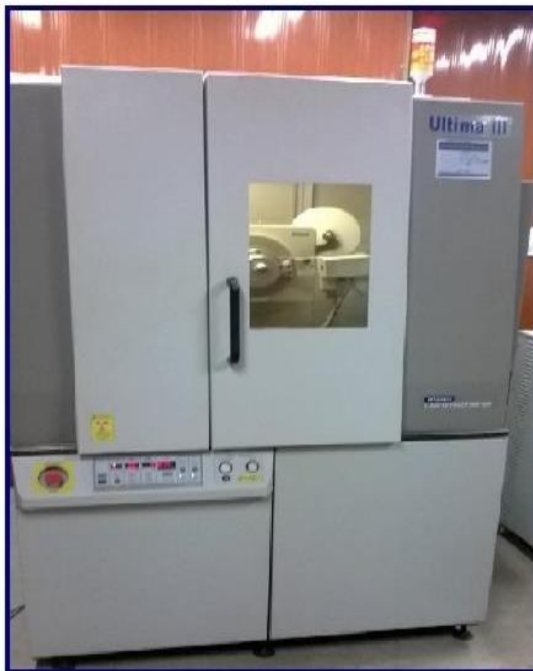
Fig. 3.9: Experimental setup of X-Ray diffractometer
