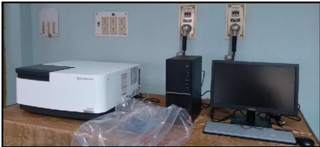
Figure 3.5: Photoluminescence analysis carried out by Horiba Jobin Yvon Fluoramax
