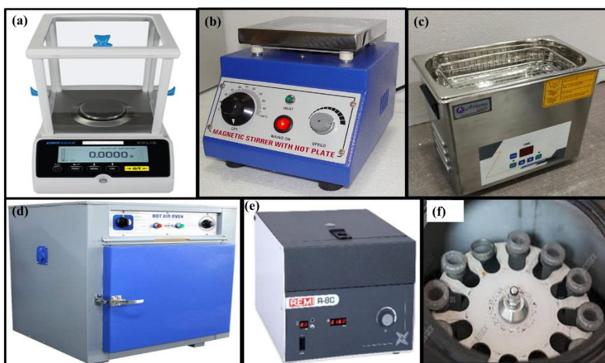
Figure 3.2: (a) Weighing Machine (b) Magnetic Stirrer (c) Sonicator (d) Hot Air Oven (e) Centrifuge Machine (f) Placement of Centrifuge tubes inside the machine
