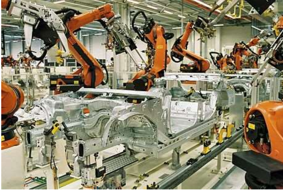
Figure 1.3. Advanced robotics in automotive production (source: Wikipedia.org)
