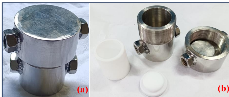
Fig. 1.19 (a) The external view of the autoclave used for the synthesis described in this thesis with Teflon inserts used as digestion bombs; (b) Different parts of the autoclave.
