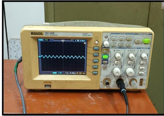
Fig. 4.10. Leakage current recording using digital storage oscilloscope (DSO).
