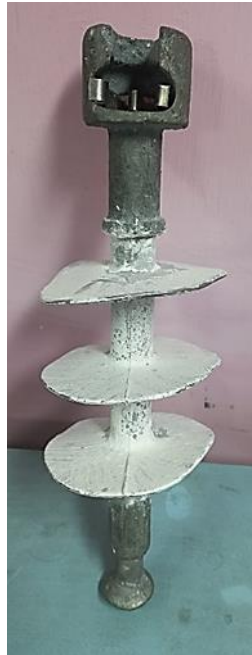
Fig. 4.4. 11 kV artificial partially contaminated Polymer Insulator
