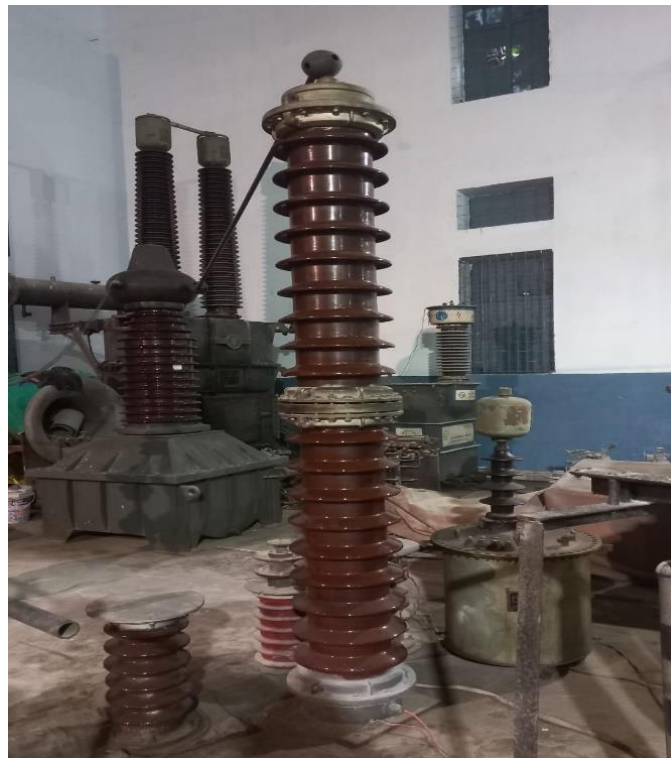
Fig. 4.6. Photograph of high voltage potential divider.
