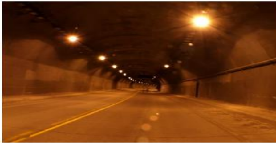
Figure 2.1.1 Example of Poor Surface Contrast
