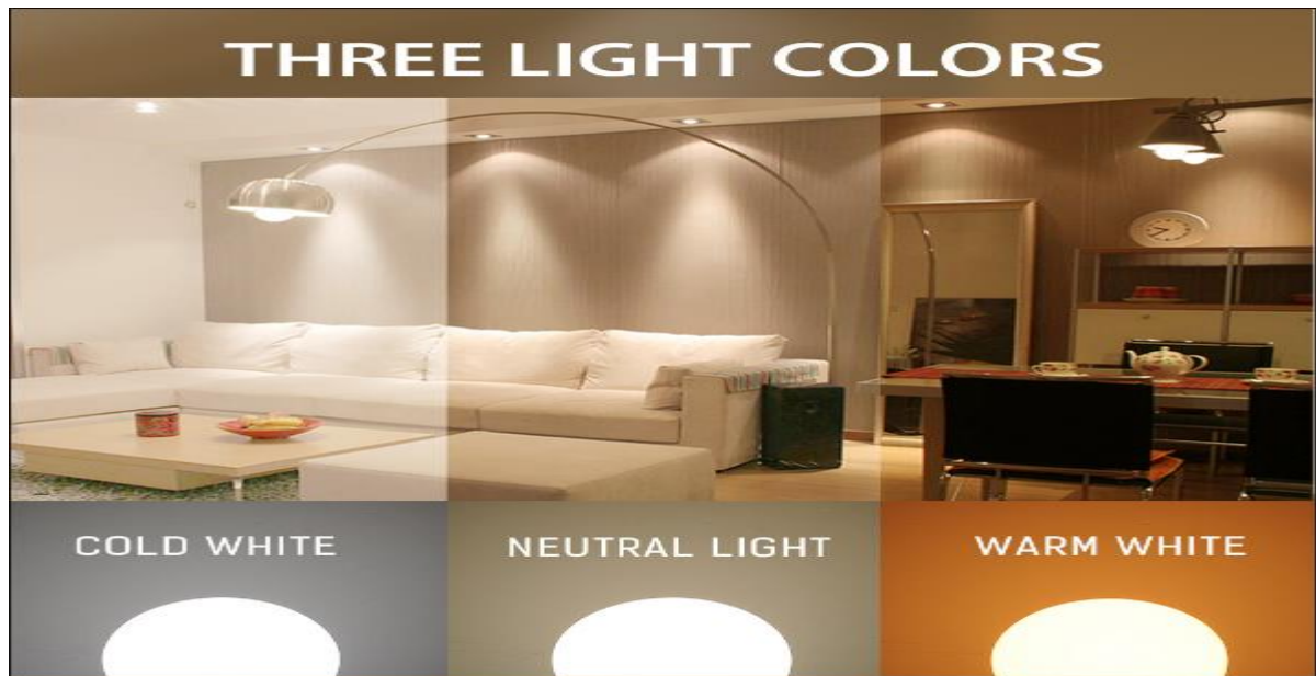
Figure 3.2 Objects under lamps with different CCT
