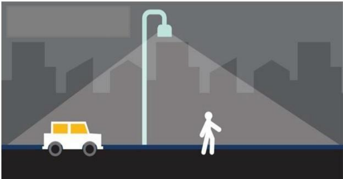
Fig.2.10: Uniform light distribution due to good optics
