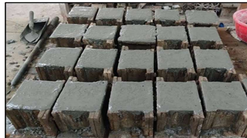
Figure 28: Mixture compacted in moulds
