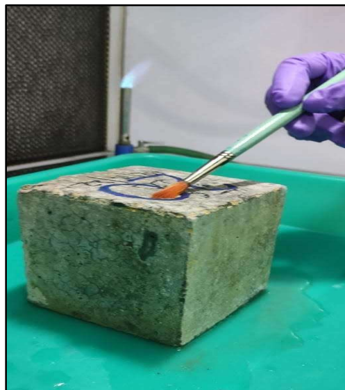
Figure 31: Applying nano silica coating in concrete surface
