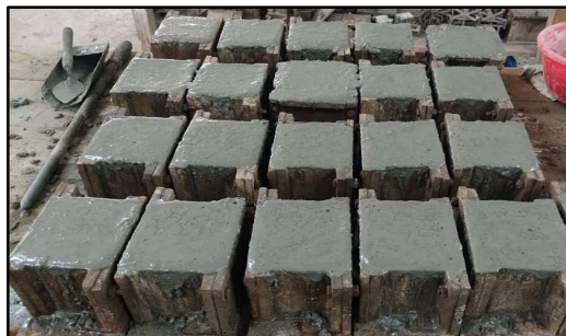
Figure 23: Mixture compacted in the moulds
