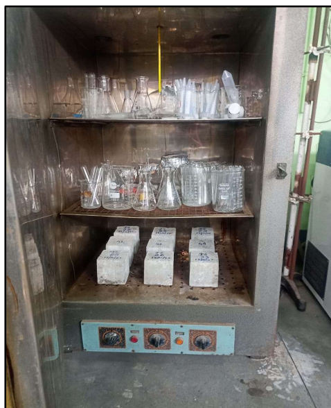
Figure 32: Drying the coated cubes in hot air oven
