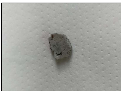
Figure 46: Chips size samples of concrete
