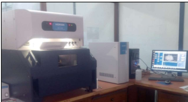
Figure 45: Energy Dispersive X-Ray Fluorescence (EDXRF) Spectrometer
