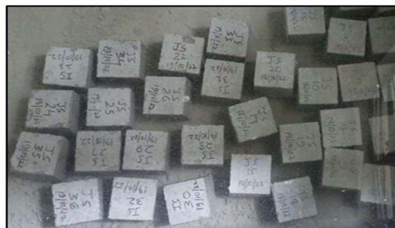
Figure 29: Curing for 28 days under water
