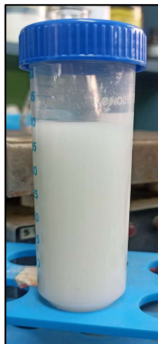
Figure 13: Combination of binder, silicon oxide nano-powder and water (Nano Silica Coating)
