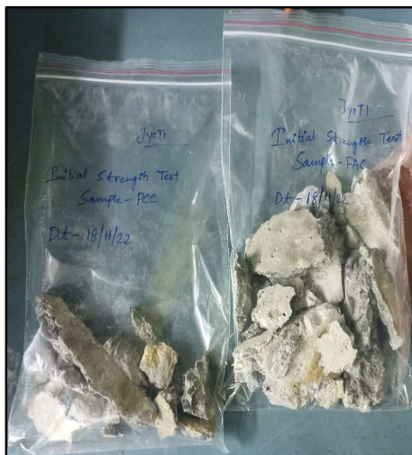
Figure 41: Small pieces of concrete cubes collected after compressive test
