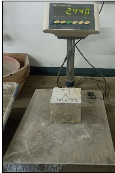
Figure 36: The weight of a concrete cube is being measured in the weight balance.
