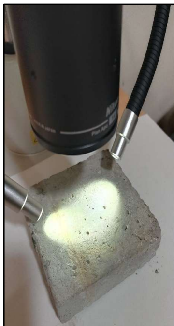
Figure 38: Concrete cube observed under the stereo microscope.
