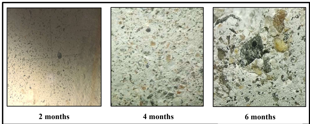
Figure 55: Stereo microscopic images of concrete cube surfaces infected by fungus from the biodeterioration set-up.
