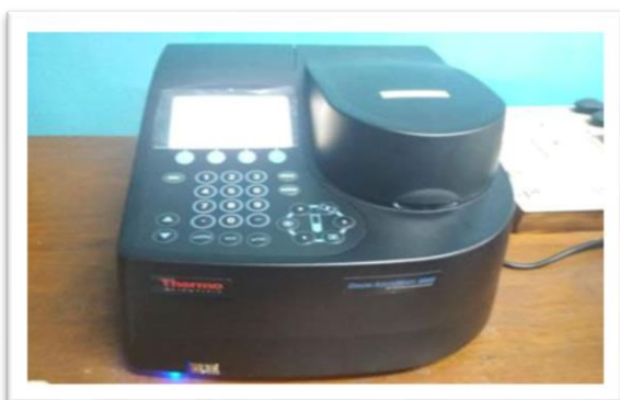
Figure 8-2: Orion Aquamate 8000 UV – VIS Spectrophotometer at 510 nm Wavelength
