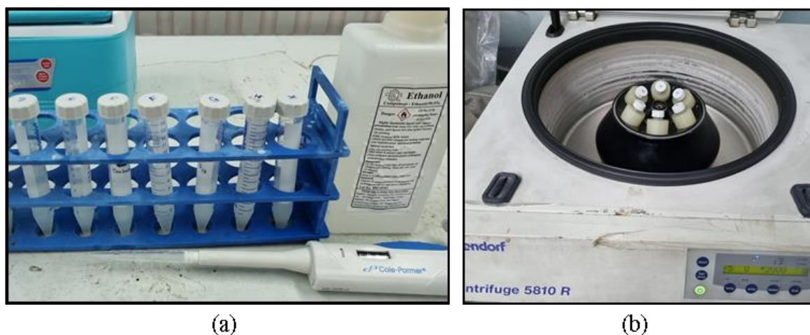
Figure 33: a) Addition of ice cold ethanol, b) Centrifugation at 2000g
