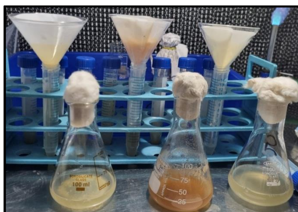
Figure 30: Cultures filtered using Whatman filter paper
