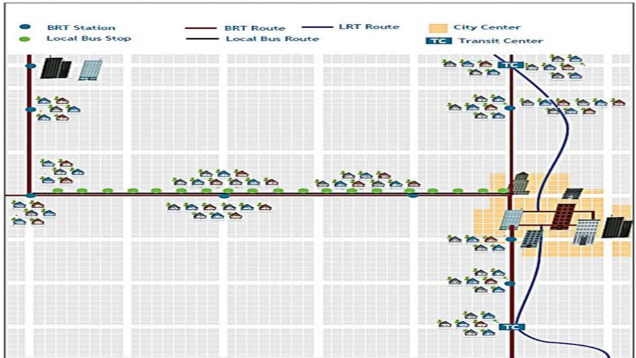
Figure 46 Typical BRT Route, Operating on Primary Arterials and Making Fewer Stops than Local Bus Service
