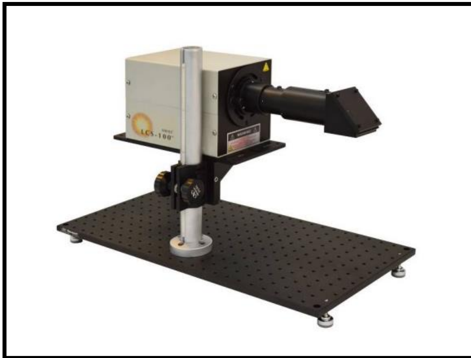
Fig 3.7: Newport LCS - 100 Solar Simulator.
