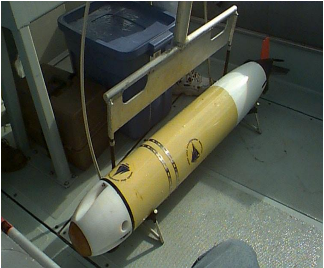
Figure 2.1 : The REMUS Autonomous Underwater Vehicle [ Prestro 2001 ]
