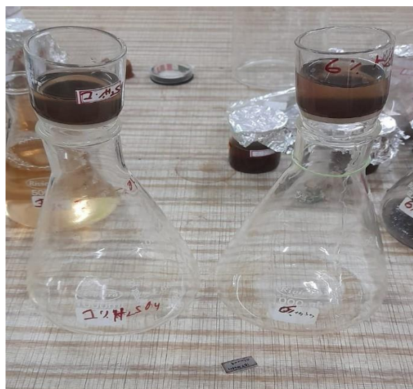
Fig 7: Insoluble lignin obtained in the crucible after washing with hot distilled water
