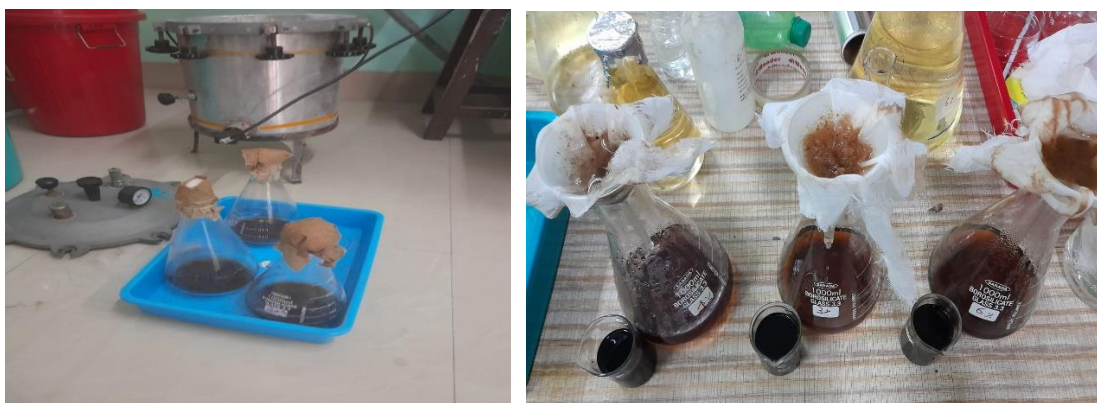
Fig 5: Experimental set up of pretreatment and the subsequent washing and separation process
