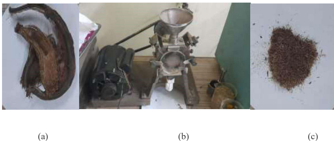
Fig 3: Raw materials, (a) Sterculia foetida , (b) Willey mill, (c) Sterculia foetida after grinding
