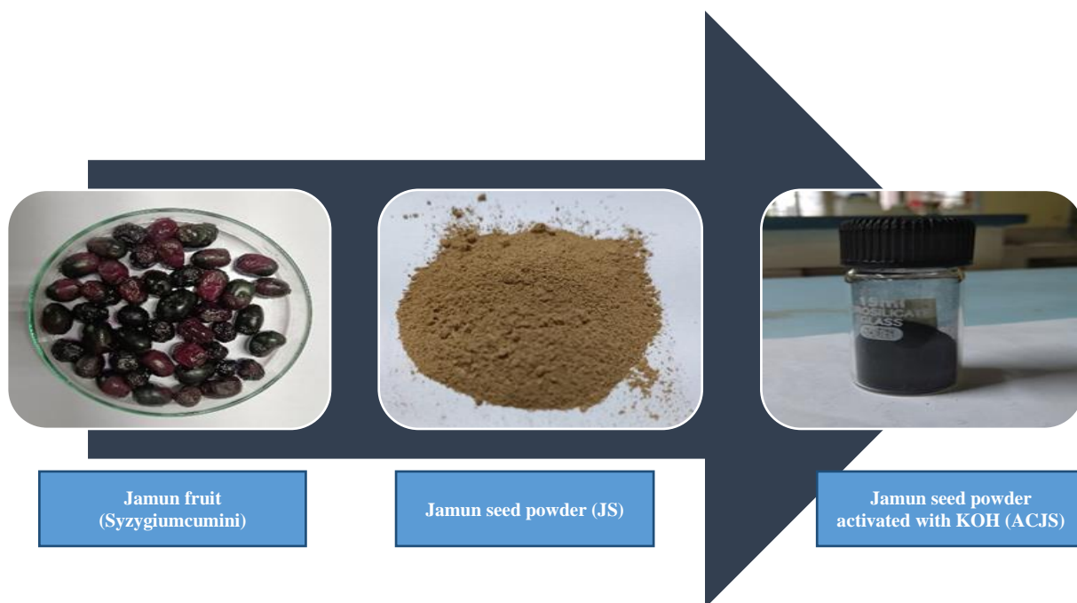
Figure 2: Experimental steps to prepare ACJS from jamun seed (JS)
