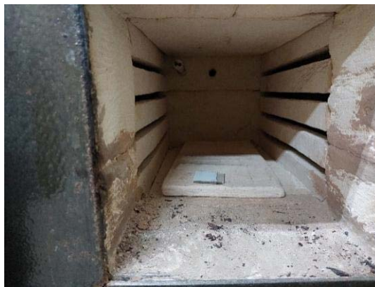
Figure 4.24 Heat treatment of \text{TiO}_2 layer inside the Muffle Furnace
