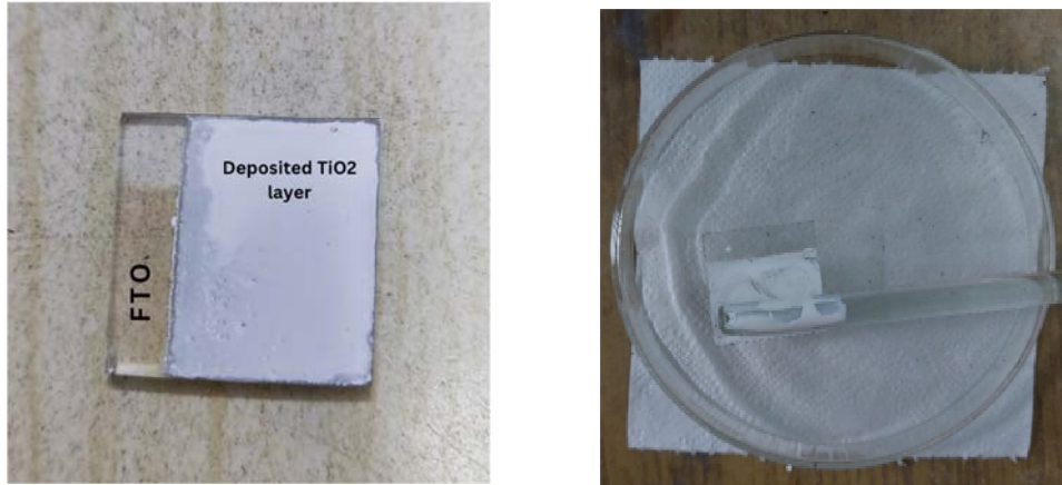
Figure 4.23 Process of \text{TiO}_2 layer using doctor blade method
