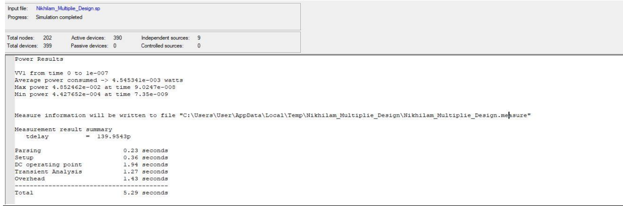
Figure 5.6 Power and Time Delay of Nikhilam Multiplier on TSPICE
