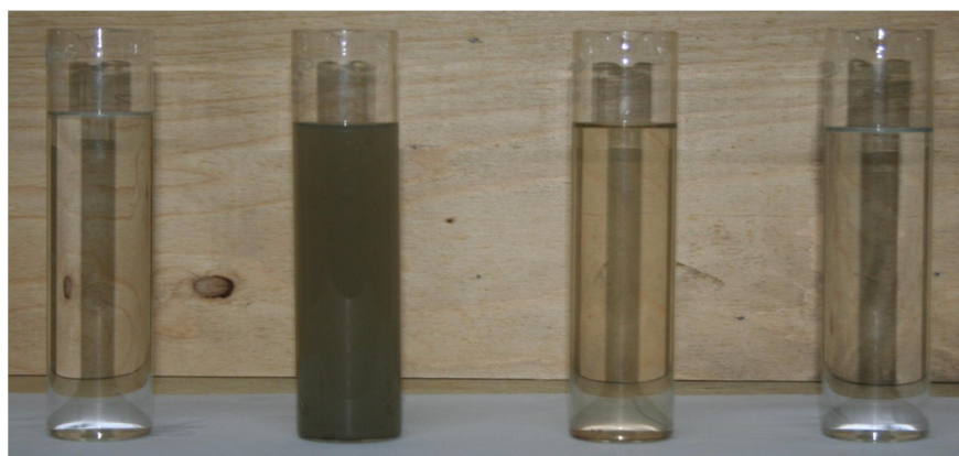
Figure 3.9 (i) MF permeate, (ii) Raw tannery, (iii) MF retentate, (iv) RO permeate
