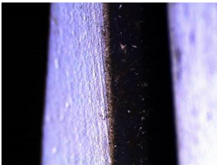
Fig. 4.5e Stereoscopic image of MnO 2 coated membrane (KM/B29/F19C/200mm/MnO 2 coated)
