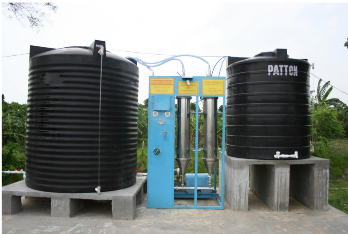
Fig 5.8 A 500 LPH capacity Ceramic Membrane plant of CSIR-CGCRI, Kolkata
