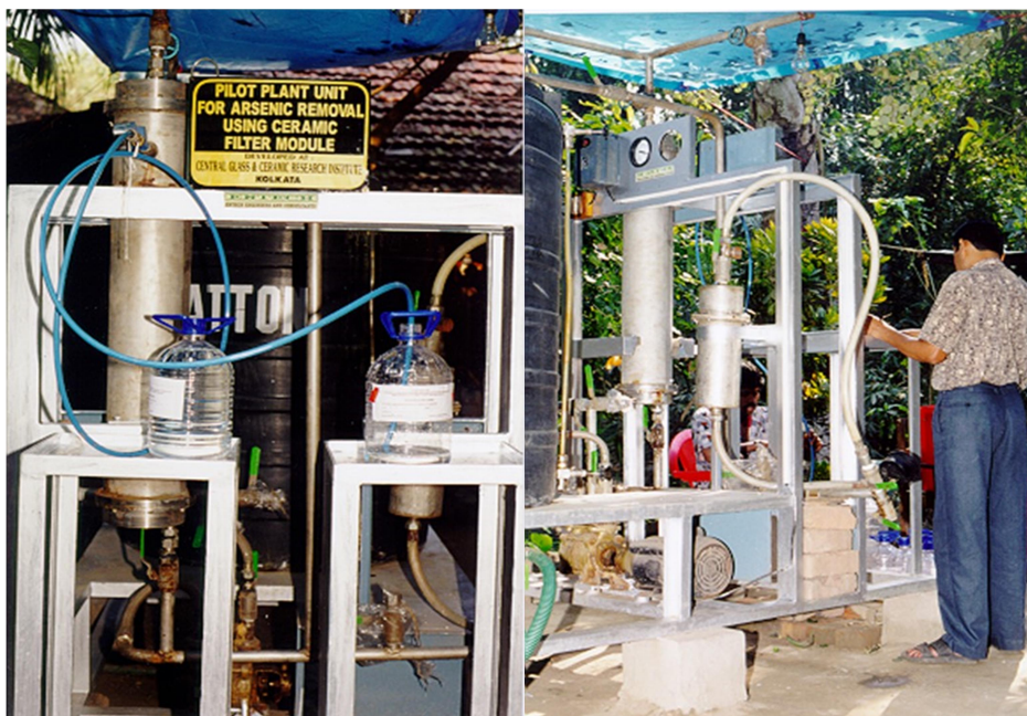
Fig 5.7 Typical SS body 60 LPH capacity test plant
