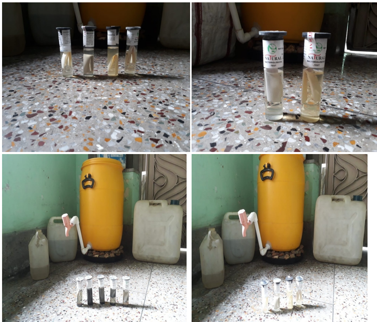
Fig.6.14 bacteriological test by H 2 S strip
