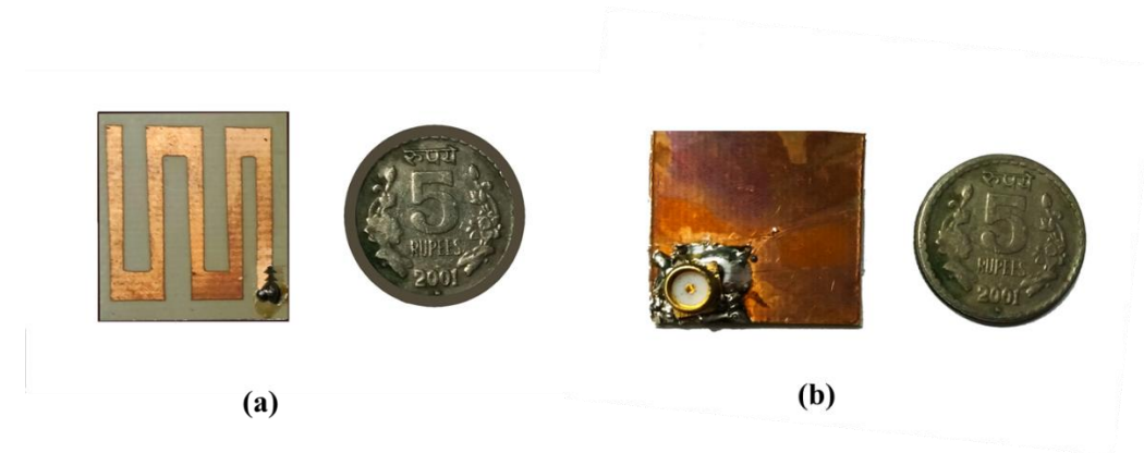
Fig. 9.8: (a) Top view (b) Bottom view of fabricated antenna
