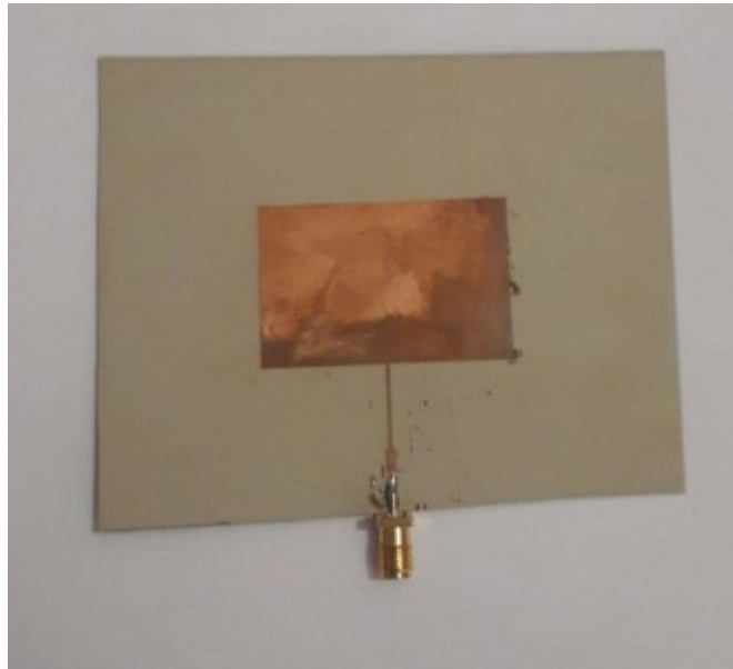
Fig. 6.1: Fabricated patch antenna with single section matching network
