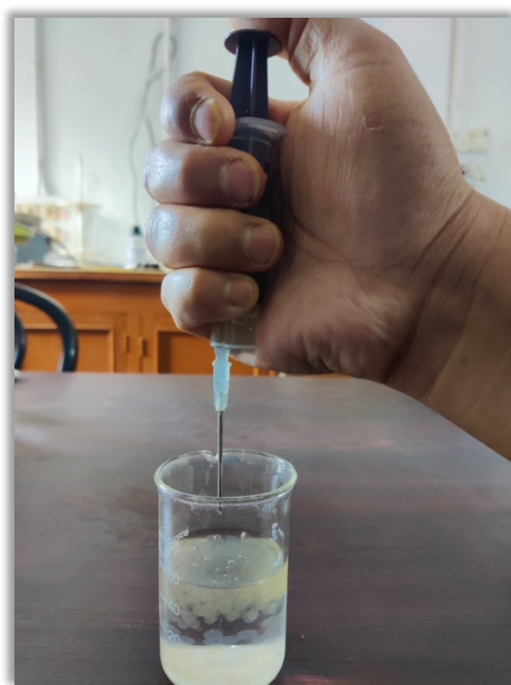
Fig. 1.3: Preparation of Calcium- Alginate crosslinked beads by Iontropic gelation method.
