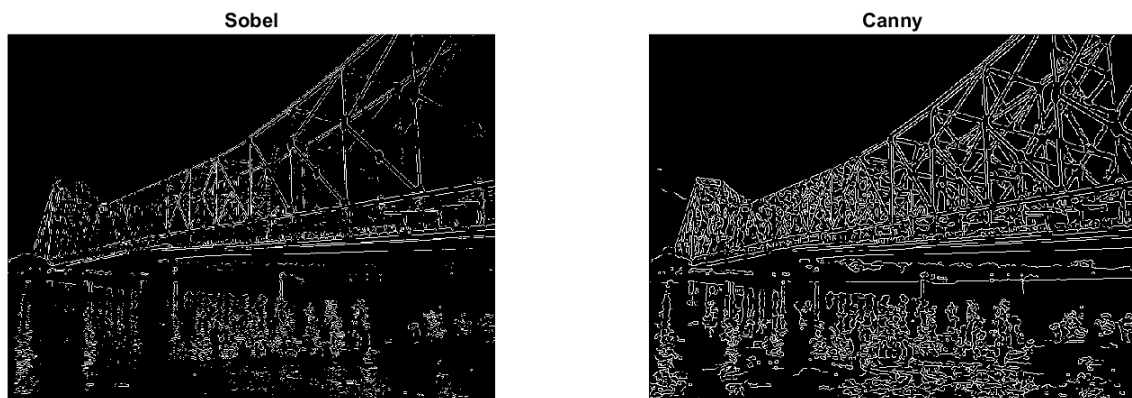
Fig 6.3 Output images of 2 edge detection operator from MATLAB for figure 6.1, Sobel (left) and Canny (right)
