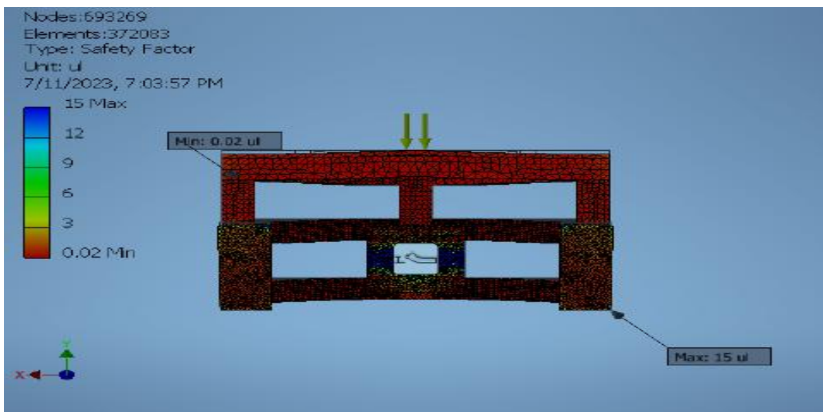
Fig. 4.2.6 (j) safety factor maximum of Carriage Fabrication
