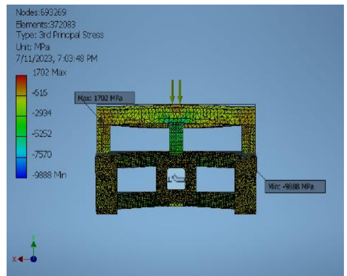
Fig. 4.2.6 (f) 3rd Principle Stress maximum of Carriage
