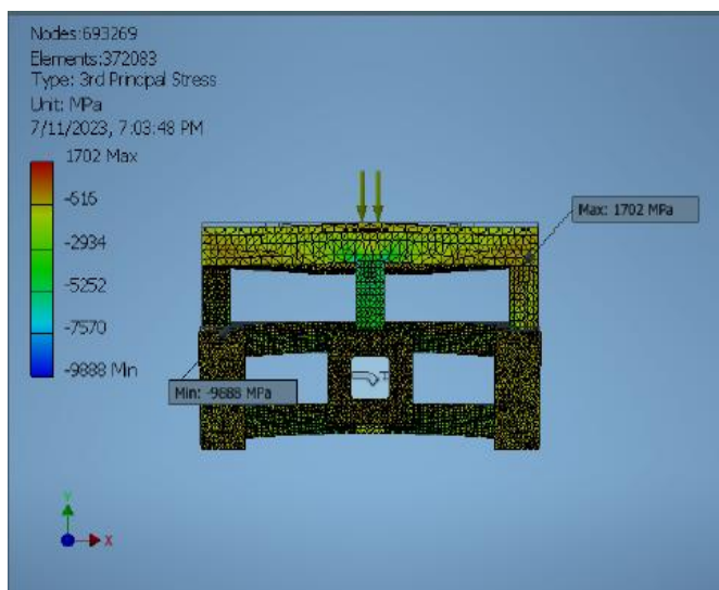
Fig. 4.2.6 (e) 3rd Principle Stress minimum of Carriage
