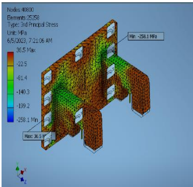
Fig. 4.2.3 (e) 3 rd Principle Stress minimum of Nut Housing Holder
