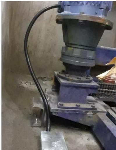
Fig. 4.3.6 additional ribbing on motor bracket
