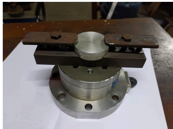
Fig.: 3.15 workpiece setup on dynamometer
