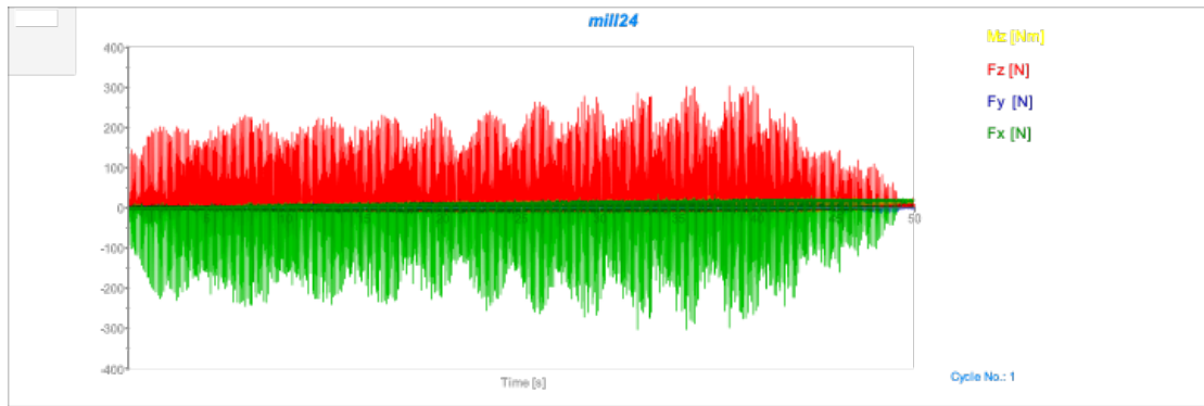
Figure 4.7: when cutting is done at high rpm
