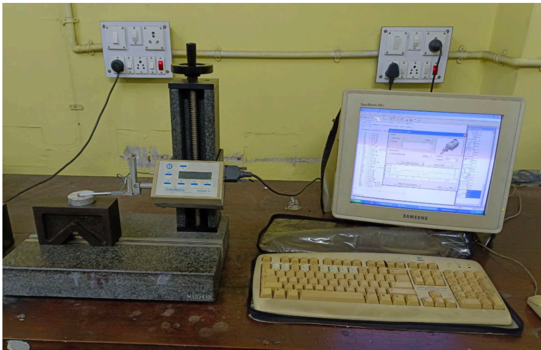
Figure 3.18 : setup for surface roughness measurement
