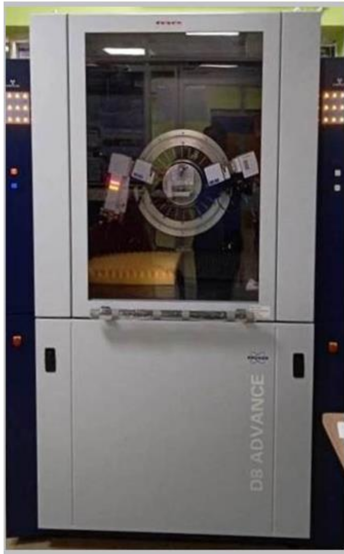
Fig. 2.5 D-8 advanced X-Ray diffraction machine, National Institute of Technology, Durgapur
