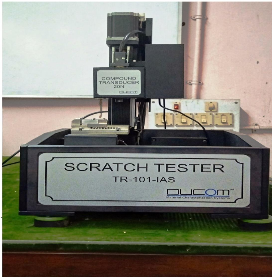
Fig. 2.6 Scratch tester (TR-101-IAS), JU M/C Elements Laboratory
