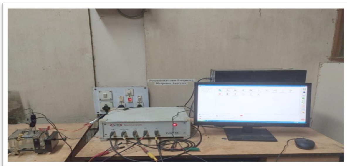
Fig. 2.7 Potentiostat from ACM Instruments Gill AC, UK
