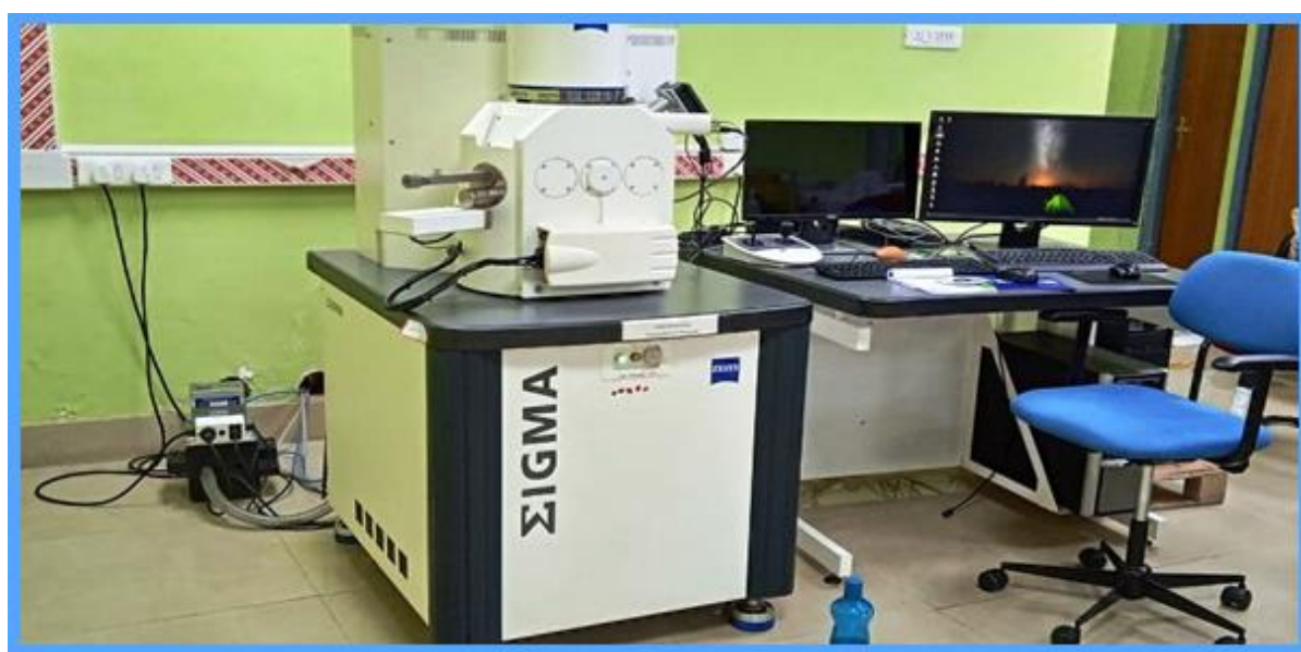
Fig. 2.3 SEM M/C1 [FESEM ZEISS, * potential - 20 kV * working distance - 9.5 mm.] National Institute of Technology, Durgapur.
