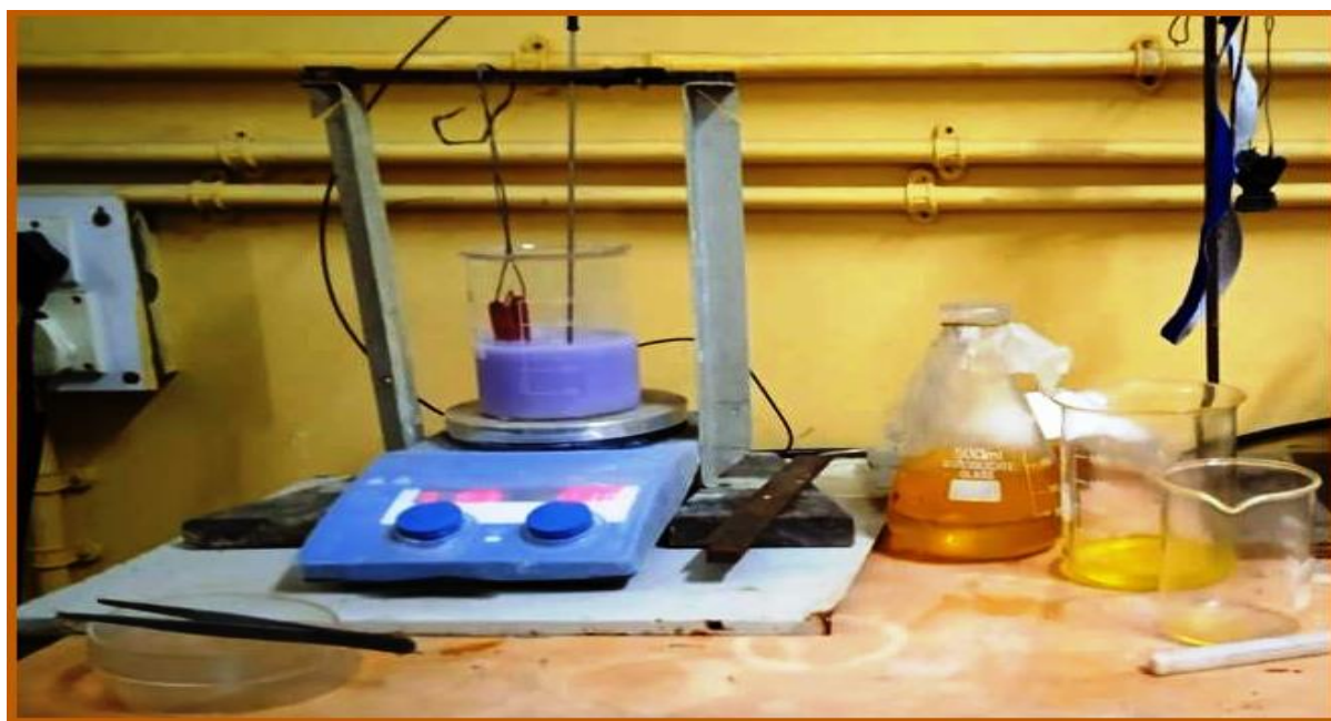
Fig. 2.2 Electroless Bath of Ni-B-TiO 2 composite coating (JU M/C Elements Laboratory)
