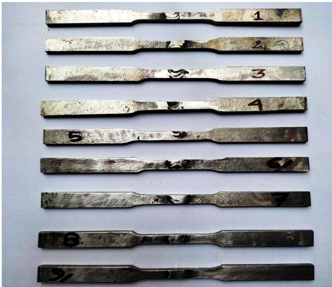
Fig. 3.14 Pictorial view of the tensile test specimen number S1 - S9
