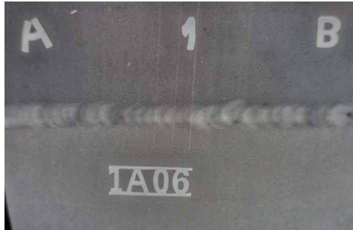
Fig. 4.1 X-ray Radiography film for sample S1
