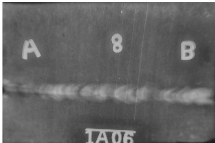
Fig. 4.8 X-ray Radiography film for sample S8
