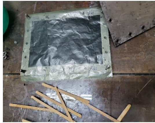
(b) Sample Preparation with Die
