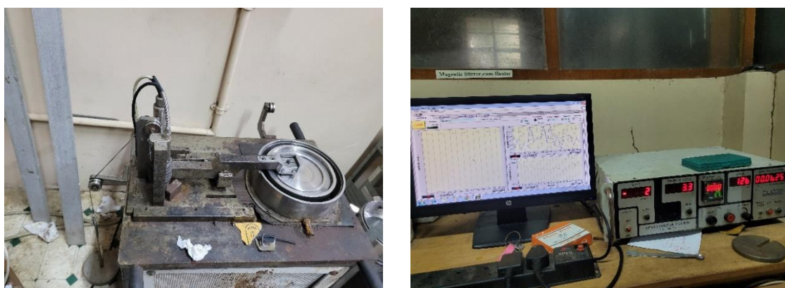
Figure 3.5. Pin-on-disc Tribo-Tester with dedicated setup.
