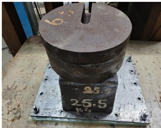
(c) Sample Preparation by compaction.
