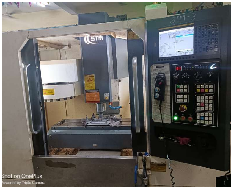
Figure 3.3: Milling Machine with FSW Tool Mounted in Tool Arbor
