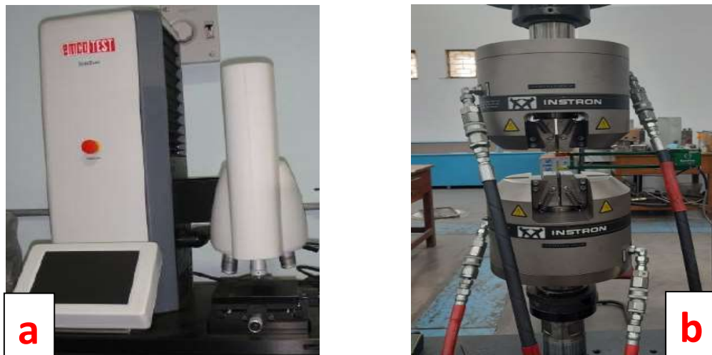
Figure 3.7: (a) Vickers Micro hardness Tester (b) Sample fitted with extensometer in INSTRON m/c
