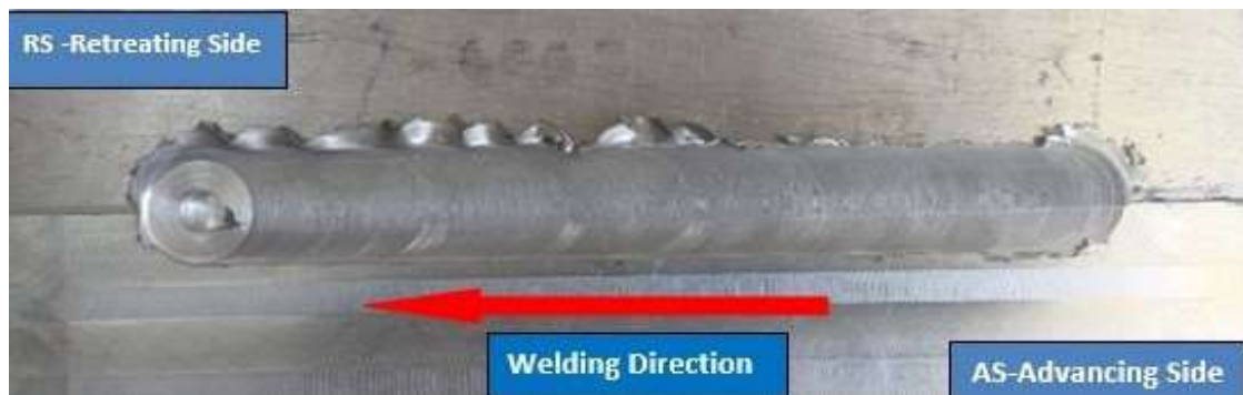
Figure 4.2: FSW welded Dissimilar Al alloys (AA 6061 & AA 6063) with RS and AS and Welding Direction.
