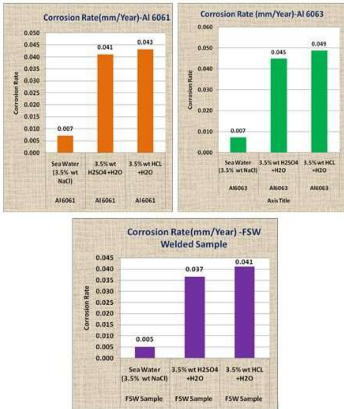
Figure 5.16: Corrosion rate Chat Base AA 6061, AA 6063 and Friction Stir welded sample with 2000 RPM Tool Rotation (a) 3.5 % HCL +H 2 O (b) H 2 SO 4 +H 2 O (C) 3.5% NaCl Solution
