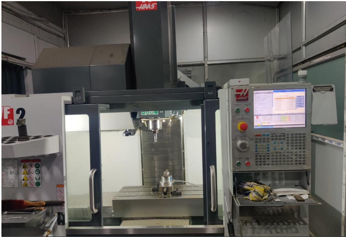
Figure 3.10 HASS CNC machine
