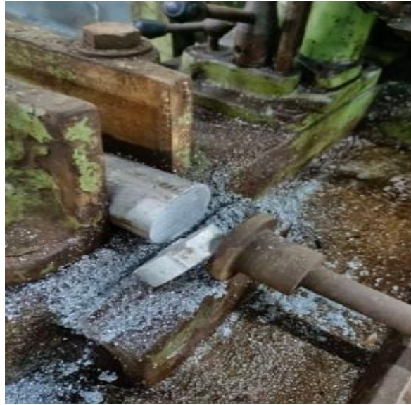
Fig. 3.2 : Cylindrical cast cut into piece
