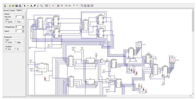
In Vivado we have implemented a single iteration of stochastic GCD circuit which is a comparator based SNG.
