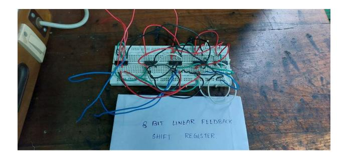
The above picture is 8-bit LFSR implemented on a bread board
