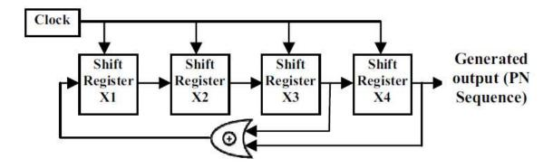
The bits in the LFSR state which influence the input are called taps. A maximum-length LFSR produces an m sequence (i.e. it cycles through all possible 2n -1 states within the shift register except the state where all bits are zero), unless it contains all zeros, in which case it will never change. The sequence of numbers generated by this method is random.
