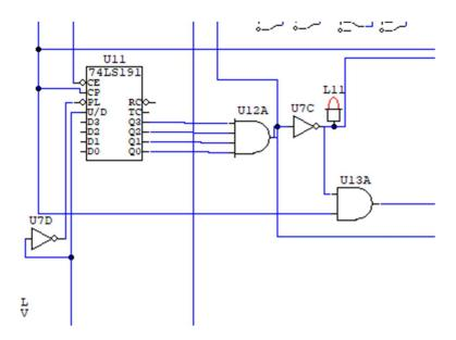
Here 74191 is a 4 bit counter which counts upto 16. Now every 16 th clock pulse the and operation of the all bits o/p is always 1. In the other words on 16 th clock pulse the NAND operation of the counter o/p always produce 0. Now if we do AND operation with clock pulse and send it to the 16 th clock pulse then SNG will skip the 16 th clock pulse and work as usual.
