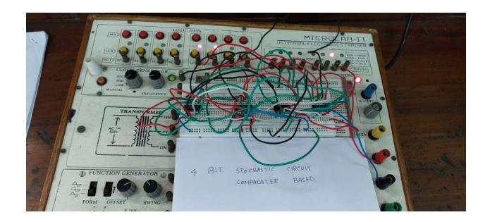
The Picture above is 4 bit stochastic number generator circuit (Comparator based ).
