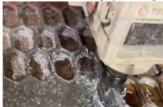
(b) Non re-entrant profile cutting
