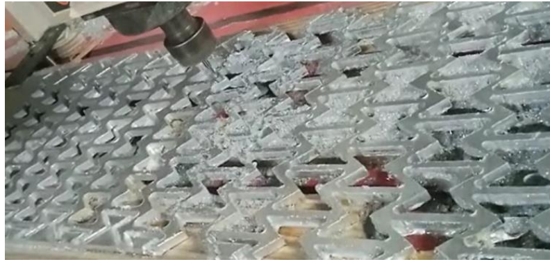
(a) Re-entrant Auxetic profile cutting
