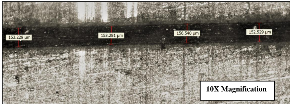
Figure 4.11 Microscopic view of Ti-6Al-4V micro-groove
