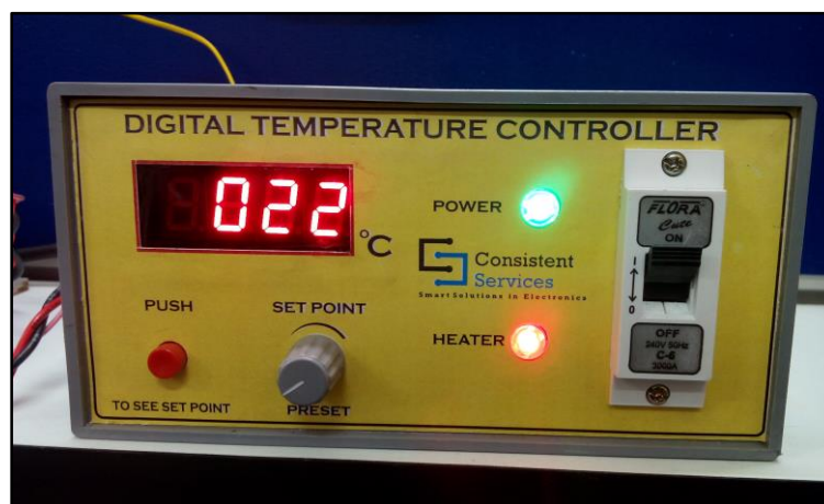
Figure 2.12 Photographic view of digital temperature controller
