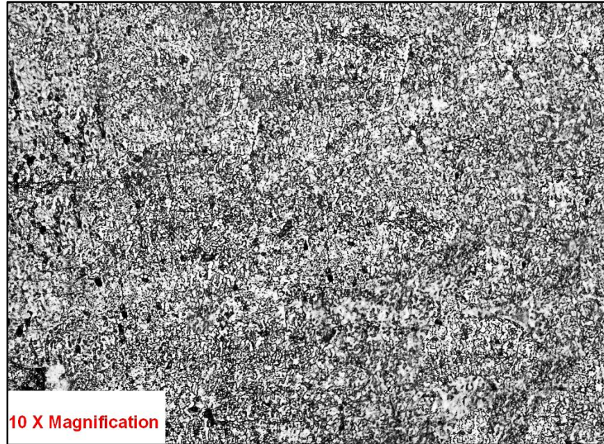
Figure 7.1 Microscopic view of an untreated surface of Hastelloy C-276 at 10X magnification
