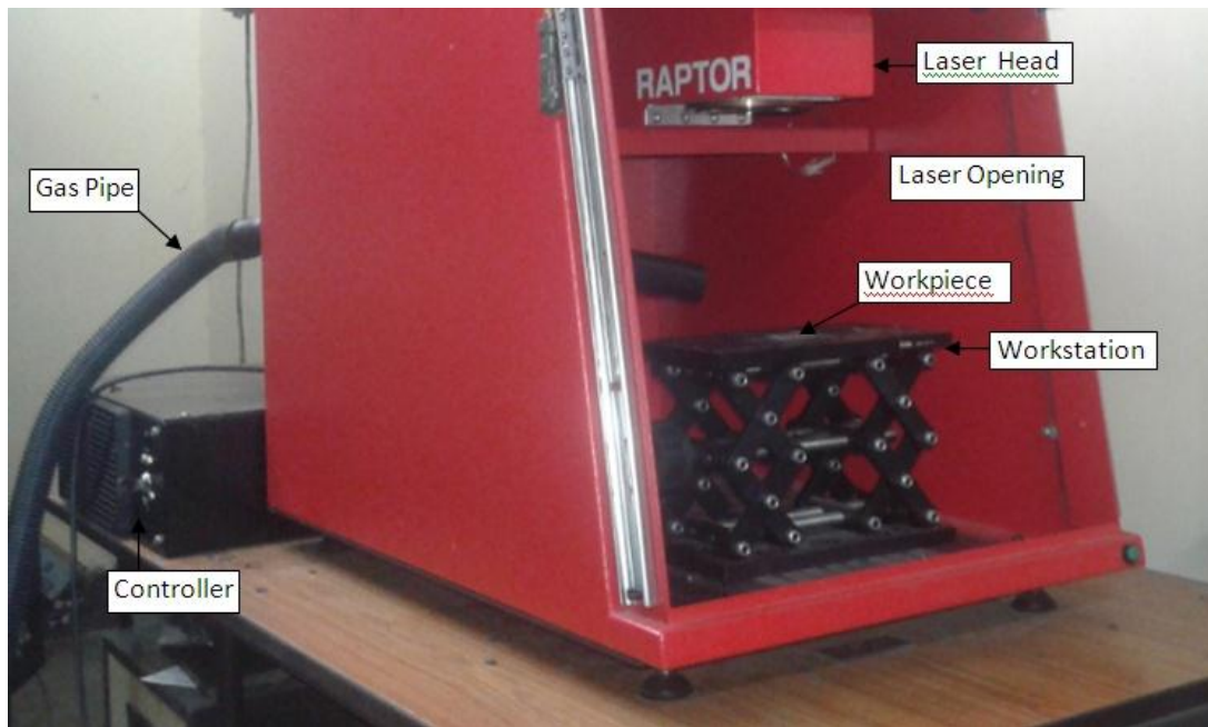
Figure 3.1 Scheme of Nd:YVO 4 Laser Set-up (School of Laser Science and Engg., JU)
