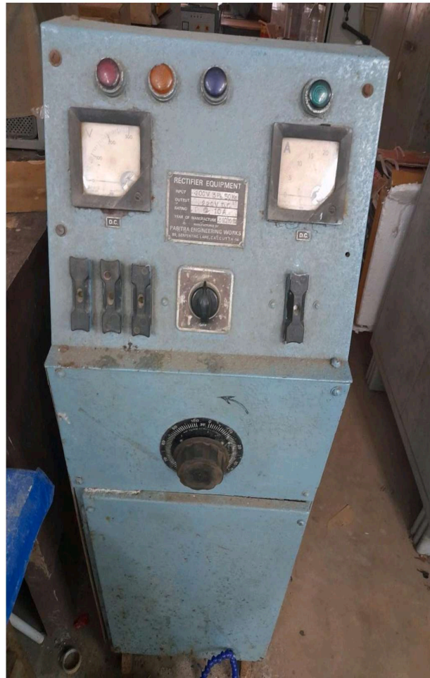
Fig:3.6 Photographic View of Power Supply Unit
