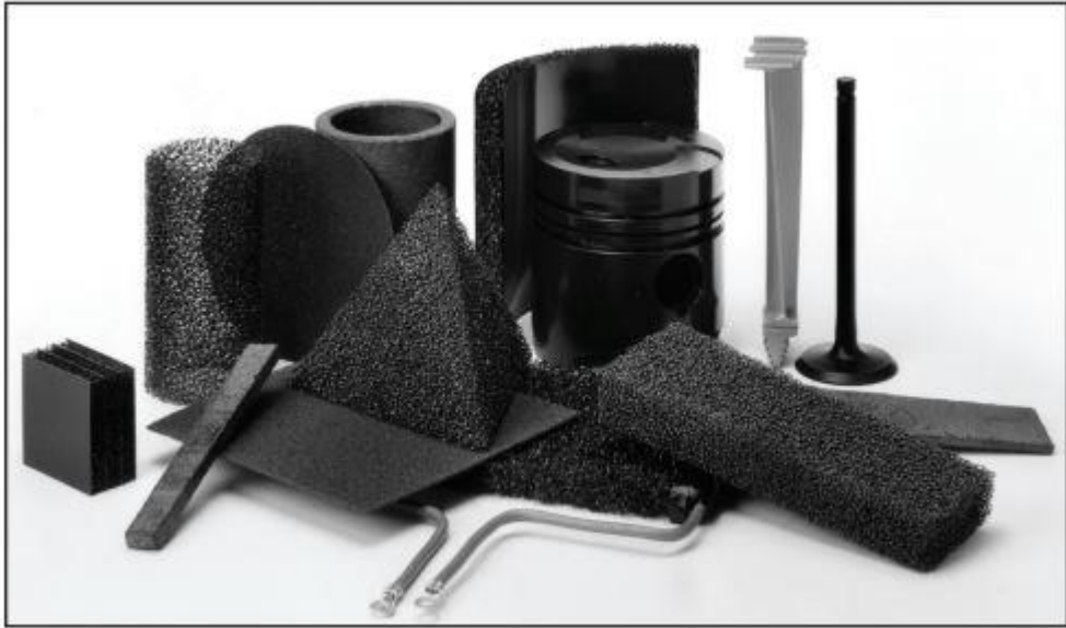
Figure 2.9. Image of SiC foams fabricated by chemical vapour deposition (CVD) of SiC on polymeric foams (Duocell ®, Auckland) [118] .
