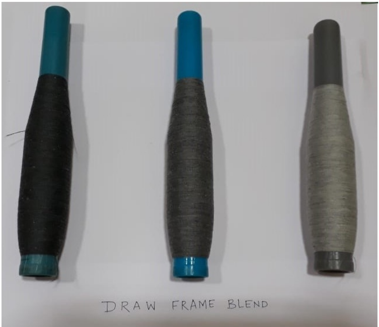
Figure 5.4 Prepared yarn samples of 20's Ne draw frame blend cotton mélangé yarn
