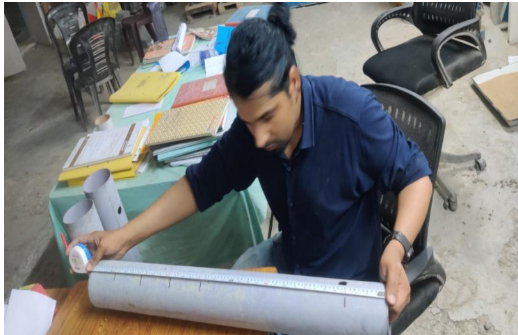
Figure 13: marking on 100 mm dia PVC test columns
