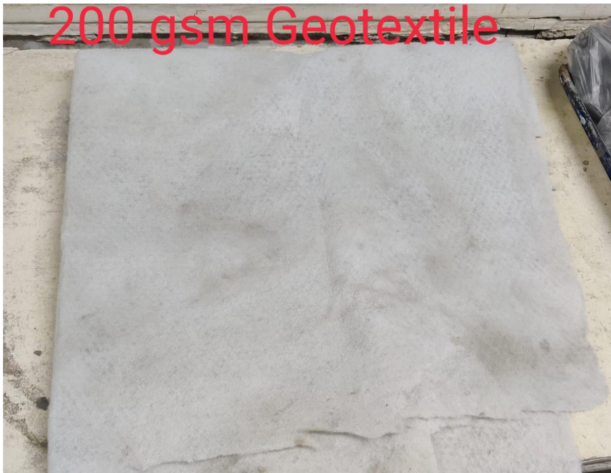
Figure 2: Sample of 200 GSM Non-Woven Needle punched Geo textile
