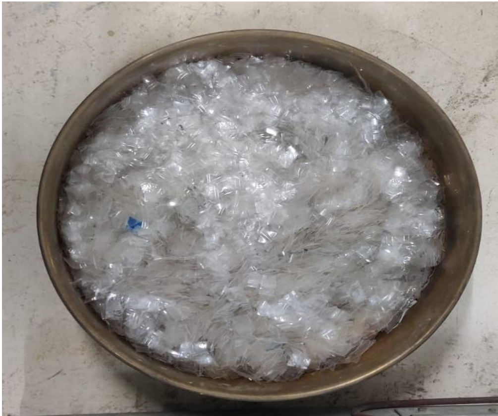
Figure 10: Graded waste PET bottle in the size range 10-4.75 mm
