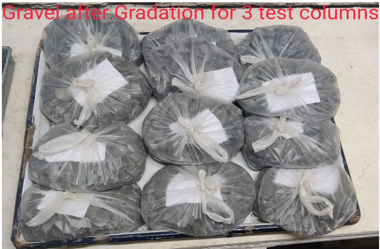
Figure 7: Gravel kept after gradation for 3 test columns (20-16 mm and 16-10 mm)
