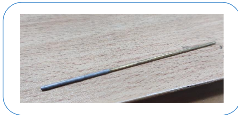
Figure 6.1: Hollow brass tool with insulated tip
