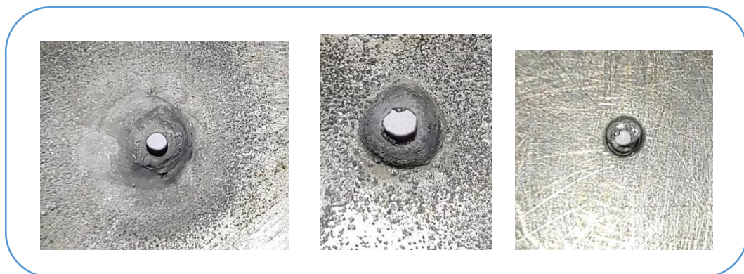
Figure 6.8: Holes drilled with low set-point current
