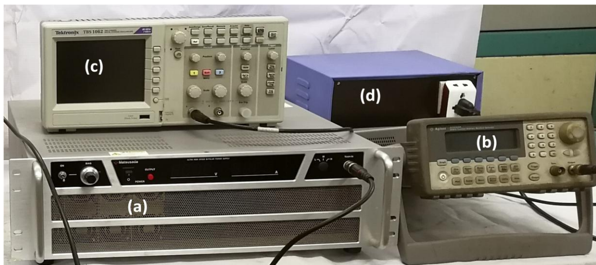
Figure 3.7: Pictorial representation of the Power Supply Unit consisting of (a) Power Supply (b) Pulse Generator (c) Digital Storage Oscilloscope (d) Transformer
